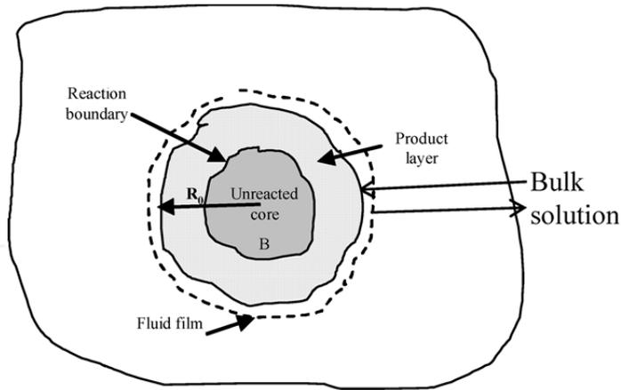
Fig. 3. Schematic diagram of shrinking core model (SCM).
