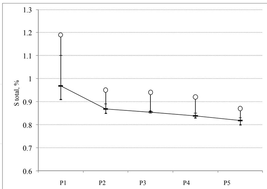
Fig. 5. Total sulfur content (%) in samples obtained from different washing steps (P1 - P5), treated by O<sub>3</sub> leaching. Initial sulfur content in original sample = 1.19 %.
